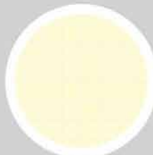
An example of contamination level to which the oil can be cleaned to (1 mg / 100 ml) NAS 7-8-9
